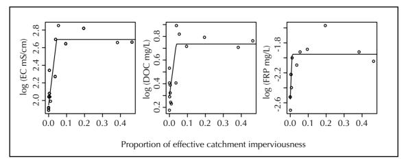
**Figure 5.** Median baseflow measurements of electrical conductivity (EC), dissolved organic carbon (DOC) and filterable reactive phosphorus (FRP) in 15 small streams in the east of Melbourne, Victoria, plotted against effective imperviousness. The trend lines show the best fit model as determined by Walsh *et al.* (in press): piecewise linear regressions to a threshold effective imperviousness beyond which there is no change.
