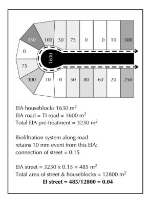
**Figure 12.** A streetscape of housing allotments with variable stormwater treatment at the allotment scale (numbers in each block = effective impervious area, EIA). A biofiltration system along the road verge retains and infiltrates water draining from the allotments and the road. Calculation of EIA and effective imperviousness (EI) of the entire streetscape is illustrated
