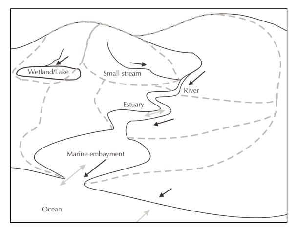
**Figure 1**. Types of receiving waters and their catchments (grey dashed boundaries). For each receiving water type, the direction of freshwater flow is indicated (black arrow), and for receiving waters with marine influence, the bi-directional nature of tidal flushing is portrayed (grey arrows).
