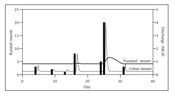
**Figure 3.** Schematic diagram showing flow response to rainfall (bars) in two hypothetical streams with a catchment of 1 km<sup>2</sup>: one draining a forested catchment (solid line) and one draining an urbanized catchment with conventional stormwater drainage systems (dashed line).
