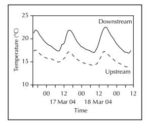
**Figure 4.** Temperature in Olinda Creek, 100 m upstream and immediately downstream of the outlet of the Hull Road constructed stormwater treatment wetland in Melbourne, measured every 5 min over three days in March 2004. The creek downstream of the wetland was 3–4°C warmer and the variation from day to night was ~1°C greater than the creek upstream (Source: Walsh 2004a)
